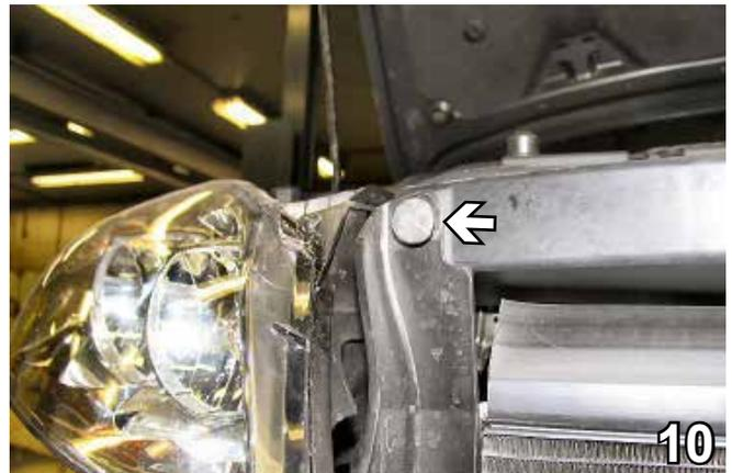
10. Remove one christmas tree push pin from upper air dam, just inside headlight assembly, both sides.
