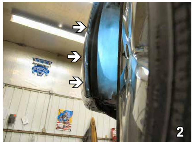
2. Remove two Christmas tree push pins and one metric bolt from the edge of wheel well, just forward of front tire with the 7MM socket, both sides.
