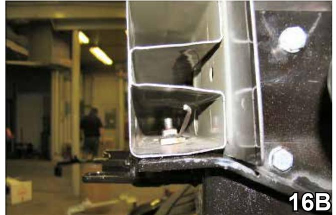
16. Using the baseplate as a template, drill a hole into the bottom of metal bumper with the 13/32" drill bit, both sides. Insert the 3/8" nut plate with the 12" wire into the open end of metal bumper to align with drilled hole, tighten 3/8-16 x 1 1/2" hex bolt and lock washer with the 9/16" socket, both sides. Be sure and use loctite red on all bolts before tightening. Tighten all bolts according to torque chart in the General Instruction sheet.
