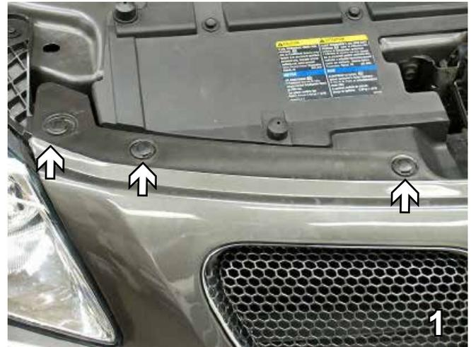
1. Remove the six push pins from the top edge of fascia just between headlight assemblies.
