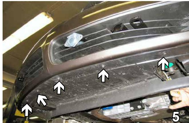
5. Remove the five metric bolts from lower edge of fascia with the 7MM socket, pull corners of fascia to the side of vehicle to release tabs, pull fascia forward and set aside.
