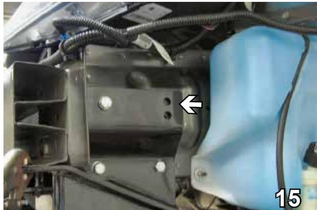
15. Slide baseplate onto the frame rail and up to bottom of metal bumper, clamp baseplate to bumper with vise grip, both sides. Align baseplate to existing bolt location for the horn bracket on the driver's side, replace and tighten existing metric bolt for horn bracket to hold baseplate in place. Be sure to align lower holes of baseplate to the center of lower frame webbing before drilling holes. Align passenger's side of baseplate to the frame to the same location as the driver's side and
